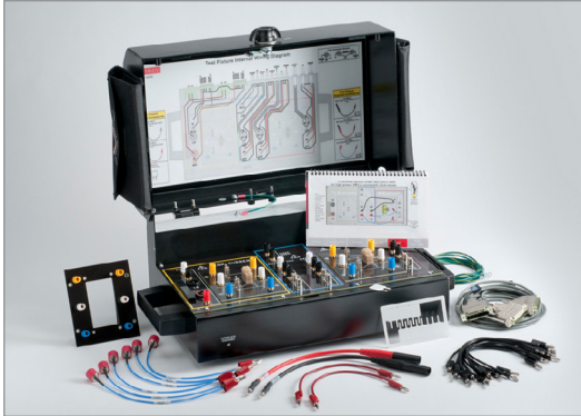
8010 High Power Device Test Fixture
