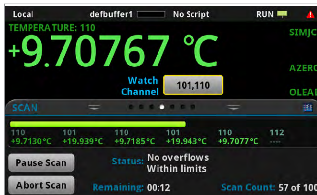
Quickly and easily monitor the status of a test using the DAQ6510 scan status screen.
